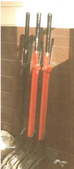
The redundant cabin and its Ground Frame were brought to Tyseley and positioned in the centre of the site adjacent to the electrical substation. Originally the track layout at Tyseley was fairly simple. The Ground Frame was used to operate a single switch (point) and two Ground Disc Signals. The levers were painted in the conventional colour scheme used by most Railway Companies:
