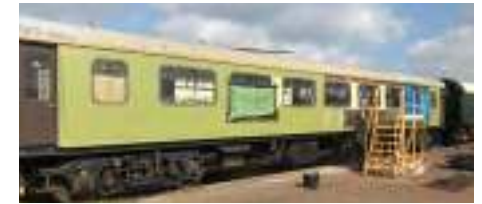
Work in progress. Pullman Parlour Car No. 353 undergoing major repairs at Tyseley. Work already completed includes removal of residual asbestos, complete electrical rewiring, renewal of internal panelling, reupholstery and recarpeting. Work is now in progress on completing bodywork repairs as seen in the photograph, complete repainting and installation of controlled emission toilets and central door locking. The car is due to enter service for the 2023 season so completing our four car 130 seat Pullman train.
