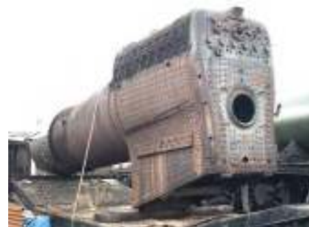
Picture: Boiler for 3840, Churchward County class 4-4-0 'County of Montgomery'
