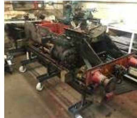
Sutton Miniature Railway 'Atlantic' Sutton Belle fully dismantled for repair and refurbishment to operating condition as funds permit. This 15” gauge locomotive was originally built for the private Hardwicke Manor Railway near Tewksbury, largely utilising Bassett Lowke designs and patterns, then moved to the SMR in 1947 where she was painted in the red livery she will be restored in. All parts are complete and work has commenced to rebuild this locomotive, but a new boiler will be required.
