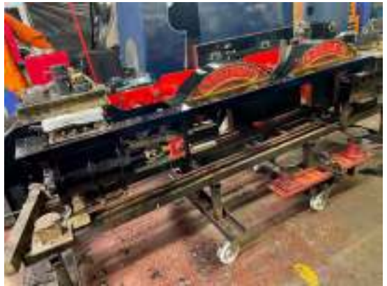
Sutton Belle – Frames and splashers stripped and repainted. Photo: Andy Watson
