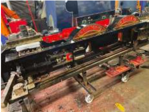
No 1: Sutton Belle – Frames and splashers stripped and repainted. Photo: Andy Walton
