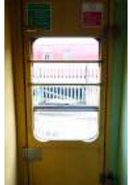
The door bars fitted to one of VT's coaches. There is still enough room for stewards to get to the door handle.
