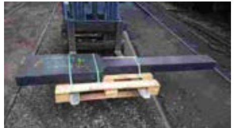
This is the block ('billet') of special steel that the replacement centre connecting rod will be machined from. Nearly 0.2 tons of steel will have to be shaved off. This will be the fourth one fitted to The Duke since 1954. (Image: Dave Oliver)
