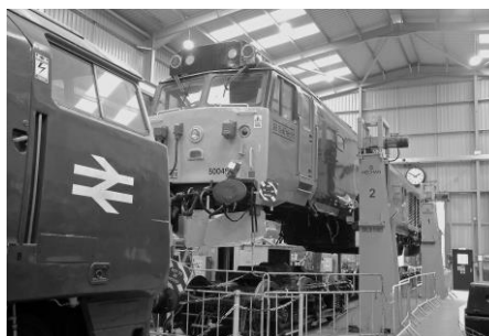
50049 on jacks in the Kidderminster Diesel Depot on 17 May 2019
