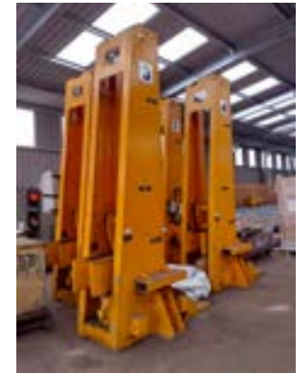
The newly arrived four Matterson 25 tonne vehicle lifting jacks pictured in the carriage shed in March 2024.
