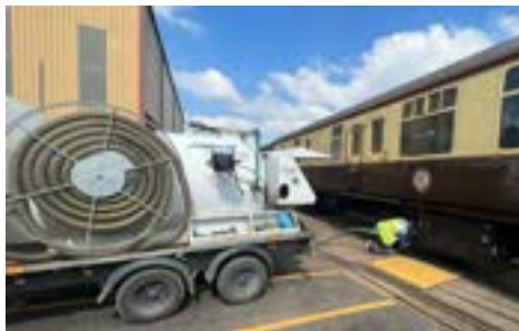
Emptying the waste tanks by vacuum pump into a bowser after the end of each journey.
