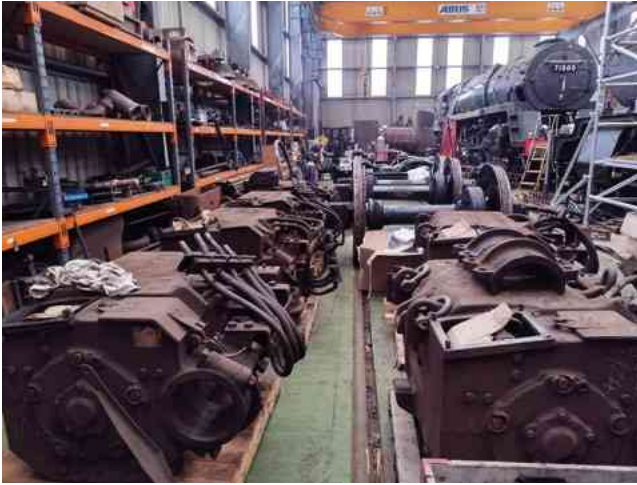
Class 37 37240 traction motors with the monoblock wheels and bogie frames in the background prior to assembly in the workshop.
