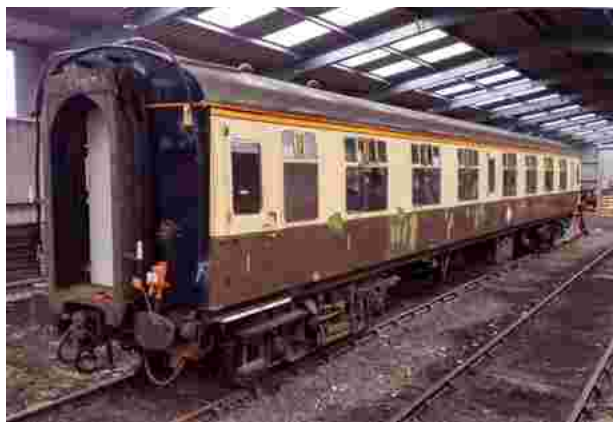
Mk1 FO no. 3141 in the Carriage Shed showing some bodyside primer application in preparation for vehicle painting.
