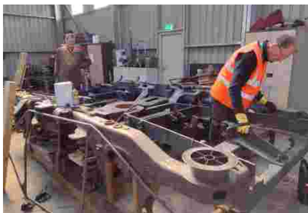
Volunteers Beresford Dickens and Ralph Sanders in the initial stages of stripping components from a Commonwealth bogie prior to clean and painting.
